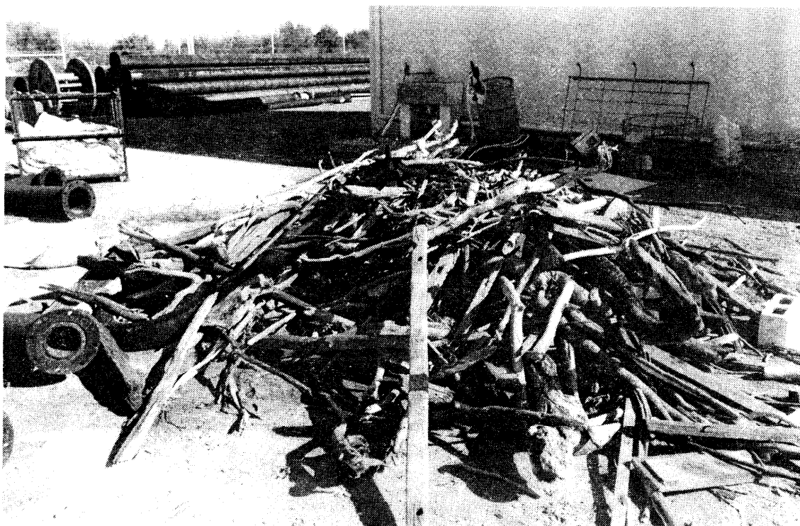
Figure 2. Debris from a single jet pump crater
