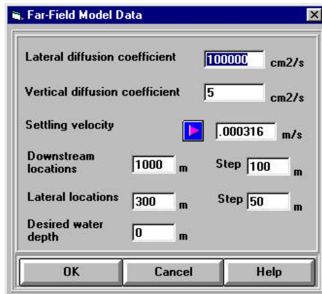
A dialog box titled "Far-Field Model Data" with several input fields and buttons. The fields are: Lateral diffusion coefficient (100000 cm2/s), Vertical diffusion coefficient (5 cm2/s), Settling velocity (0.000316 m/s), Downstream locations (1000 m) and Step (100 m), Lateral locations (300 m) and Step (50 m), and Desired water depth (0 m). Buttons for OK, Cancel, and Help are at the bottom.
