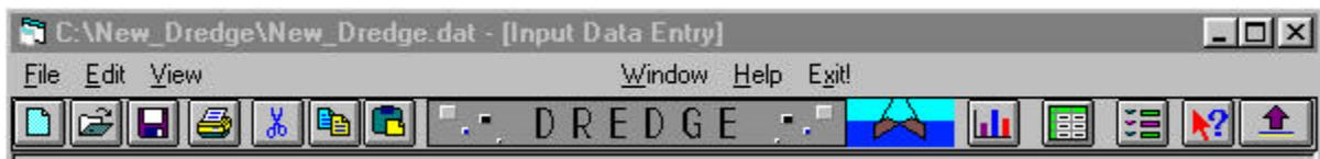
The button bar provides direct access to the most commonly used menu items. An icon on each button suggests the action that results from pressing the button; allowing the mouse pointer to hover over the button momentarily will display a tool-tip description. Pressing the left mouse button while the pointer is over the rectangular area of the button initiates the associated action. Table 2 describes the available buttons and the associated actions.
