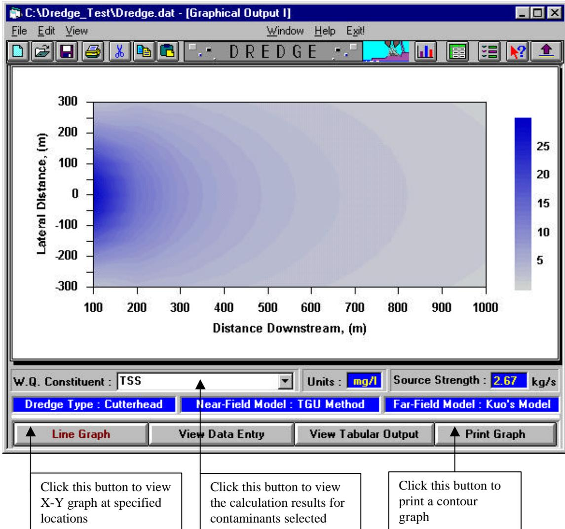
The default graph is a contour graph in which the concentration ranges are displayed using a gradually varying color bar. The user can reformat the graph by pressing the right mouse
