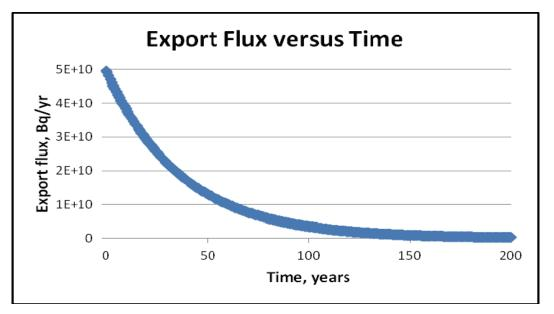
Figure 2. TREECS<sup>™</sup>-computed watershed export flux to surface water of <sup>90</sup>Sr versus time for baseline conditions (time zero is year 2000)
