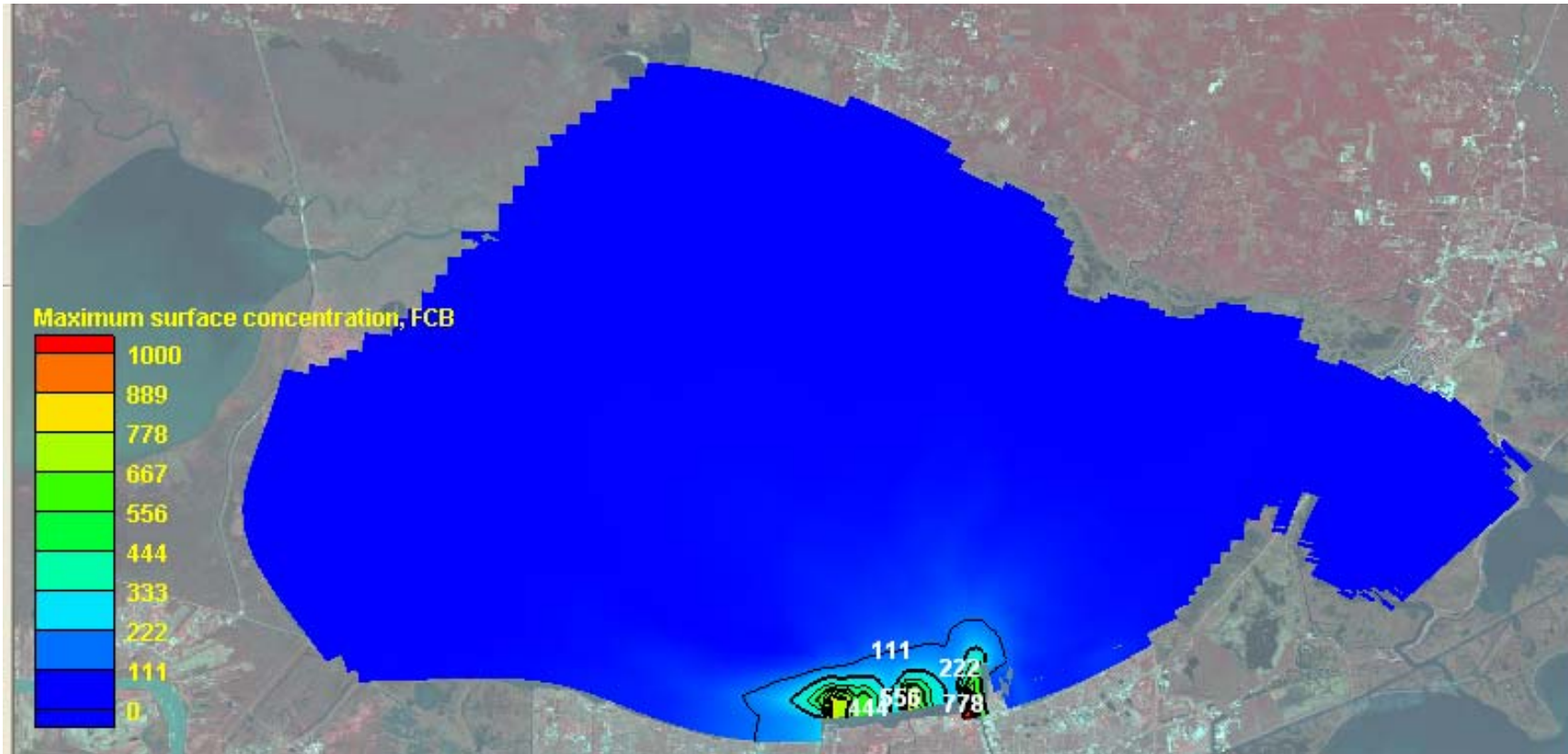
Figure A5. Incremental maximum FCB water surface concentrations (cfu/100ml) in Lake Pontchartrain for actual conditions, median loading concentrations.
