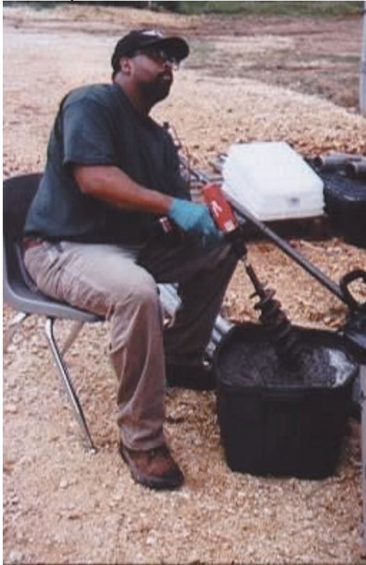
Homogenizing a composited sediment sample using a mechanical mixer
