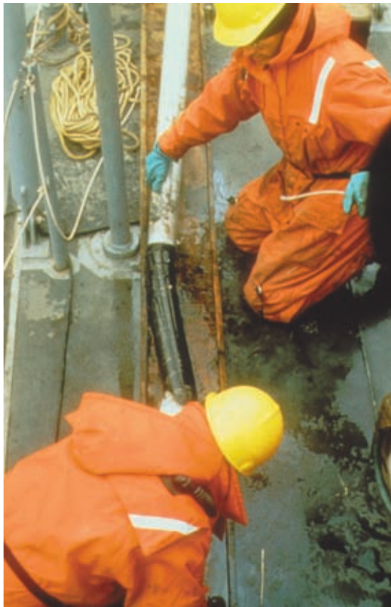
Vibracorer in use showing extrusion of the core sample for inspection and Subsampling.
