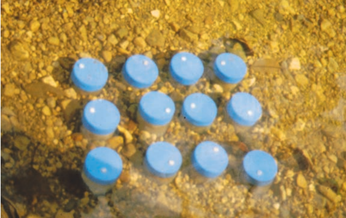
Peepers deployed in the field
