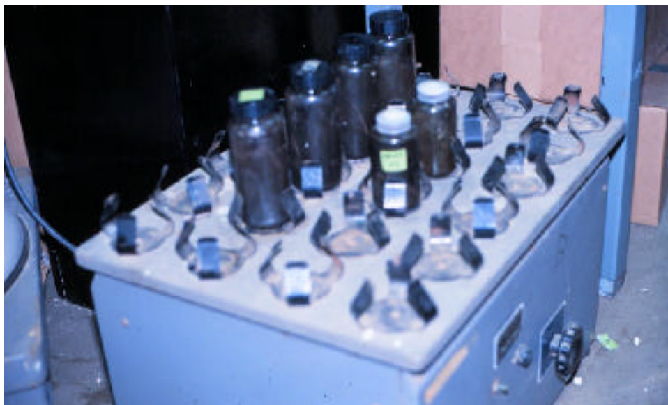
Figure 6-4. Photo of Sequential Batch Leachate Test setup
