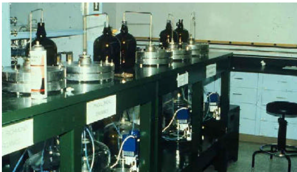
Figure 6-5. Photo of Pancake Column Leach Test setup
