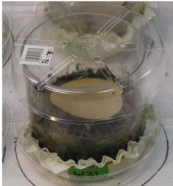
Figure 8-2. Photo of the animal uptake bioassay setup
