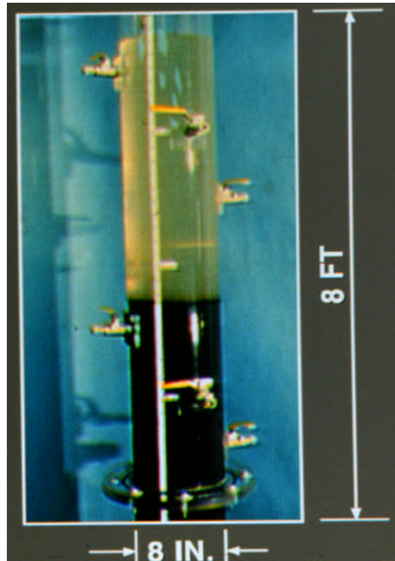
Figure 4-3. Photo of 8-inch settling column test
