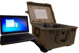
The development and evaluation of the trunnion rod test system provides the Navigation program with a tool to assist the districts in further evaluating the condition of trunion rods at dam sites.
