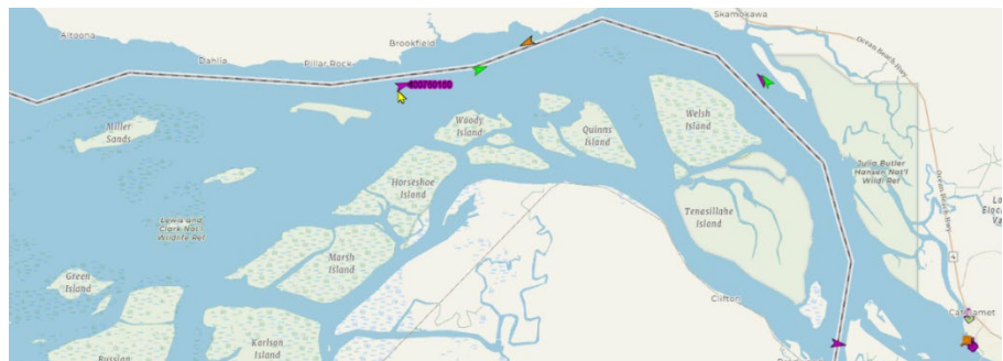
Figure 2. Screenshot from an animated playback video showing multiple vessel positions changing through the time and area of interest. Vessels are shown as triangles, color varies based on vessel information included in the AIS message.
