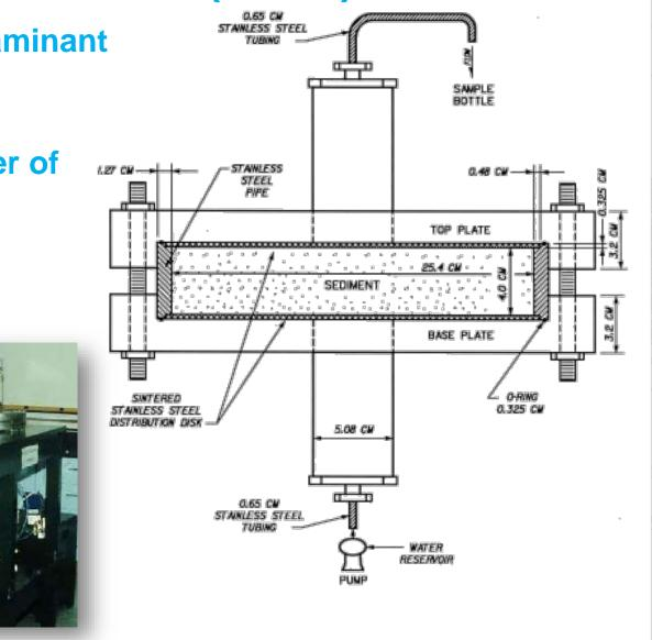
• Laboratory-scale physical model of contaminant elution from dredged material
