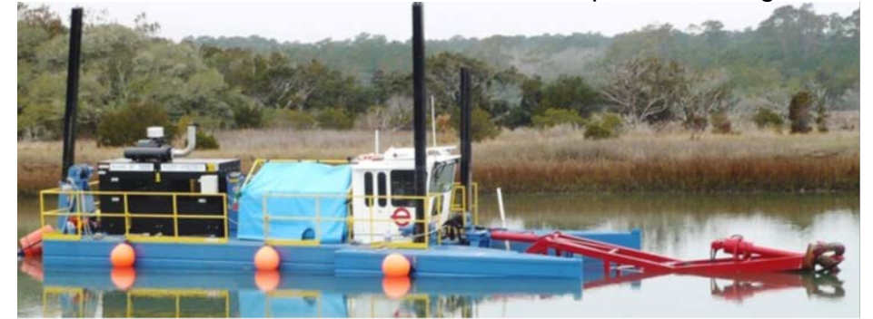
10 inch diameter discharge Ellicott 470 SL
