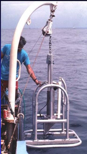
Measuring sediment deposition with Sediment Profiling Camera
