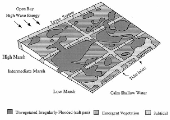
Figure 5. Recommended created marsh design. Schematic diagram of a created marsh complex consisting of adjoining hydrologically linked marsh cells. The natural marsh template for this model had a surface slope of approximately 0.04%, over a horizontal distance of approximately 600 m.
