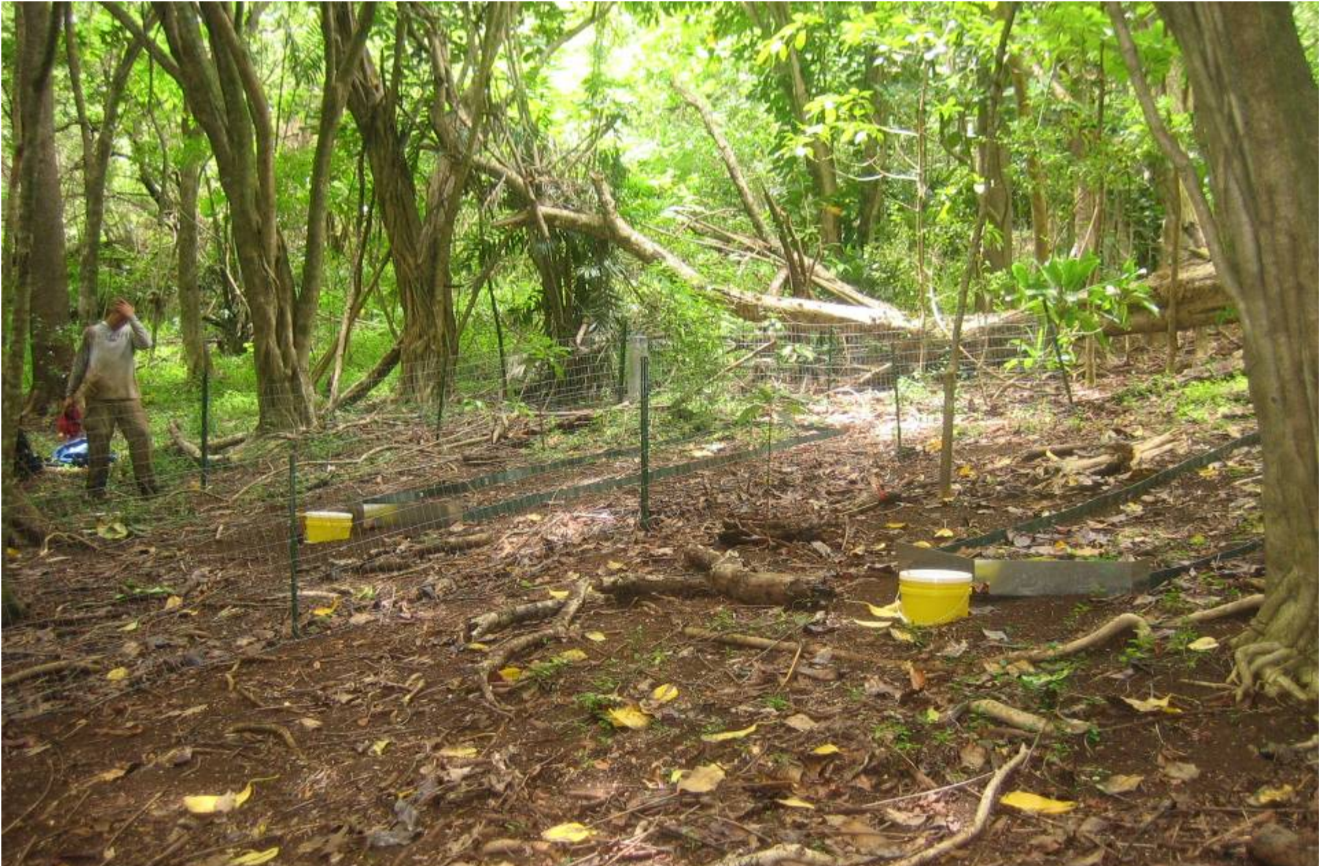
Fenced and unfenced runoff plots to study water quality impacts of feral pigs. Roundtop site, Manoa, (Browning, Bruland, Evensen, 2008)
