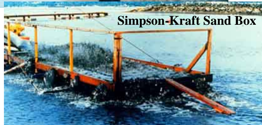
Sprayed slurry system placing sand at Soda Lake, WY
