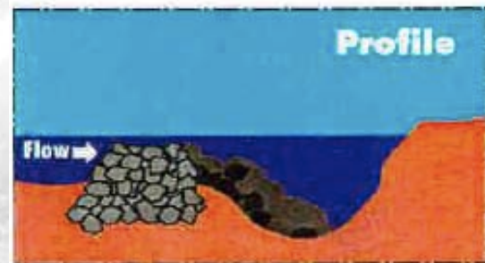
Figure 5.10. Blunt Nosed Chevron
