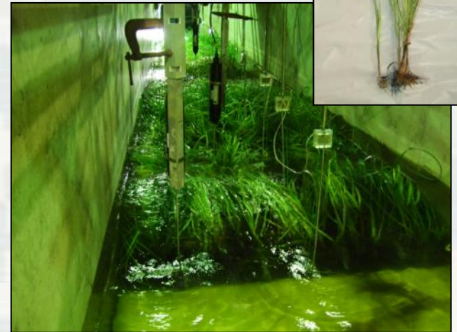
Wave attenuation by vegetation flume experiment
